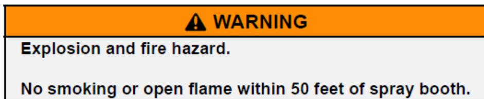
**DO NOT STORE FLAMMABLE LIQUIDS ADJACENT TO OR INSIDE SPRAY BOOTH. READ ALL PRODUCT LABELS AND INSTRUCTIONS. DO NOT USE ANY ELECTRIC POWERED AIRLESS SPRAY RIGS, PRESSURE WASHERS OR SIMILAR EQUIPMENT WHEN APPLYING A LOWFLASH POINT SOLVENT OR PEEL COATING. RUN SPRAY BOOTH EXHAUST FAN TO PURGE DANGEROUS VAPORS THAT COULD IGNITE OR EXPLODE WHILE CLEANING OR PERFORMING MAINTENANCE INSIDE SPRAY BOOTH.**
